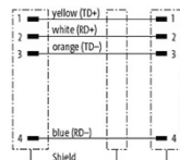
CAT 5e SF-UTP Profinet type B 1x4x22AWG PUR – Connectors: M12 D coded, RJ45
